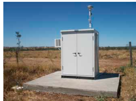
Above left: An air quality monitoring station will regularly check air quality in and around the mine site. Above right: Blast monitoring stations will be installed to measure ground vibration.
